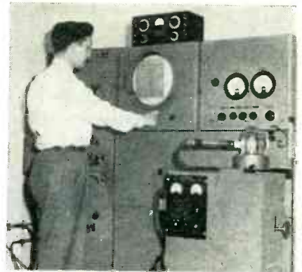
Spectroradiometer is adjusted by its designer, Austin E. Hardy, 27-year old head of the Physical Testing Lab. at RCA's Lancaster plant
