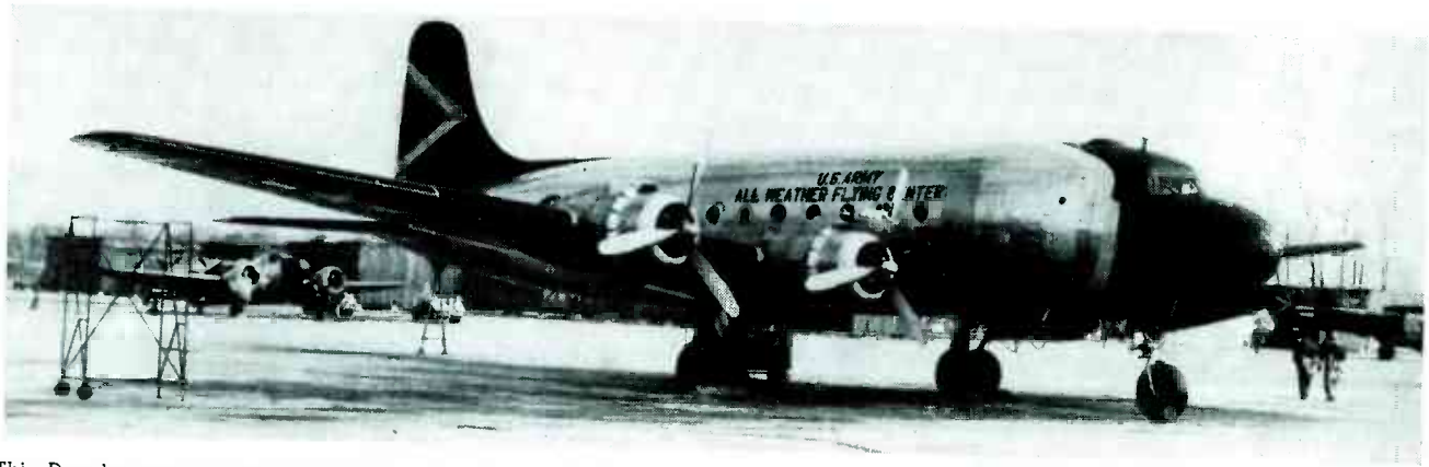
This Douglas transport flew across the Atlantic and back without a pilot at the controls. Flights between its Ohio base and Newfoundland were also automatic and nonstop, making a total round-trip flight of 8,000 miles
