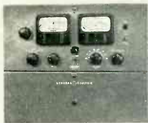
FM Station Monitor —one unit, for complete and continuous FM monitoring, plus proof-of-performance tests.
