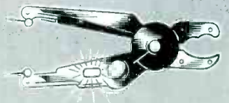
Fuse puller with built-in glow lamp as tester
